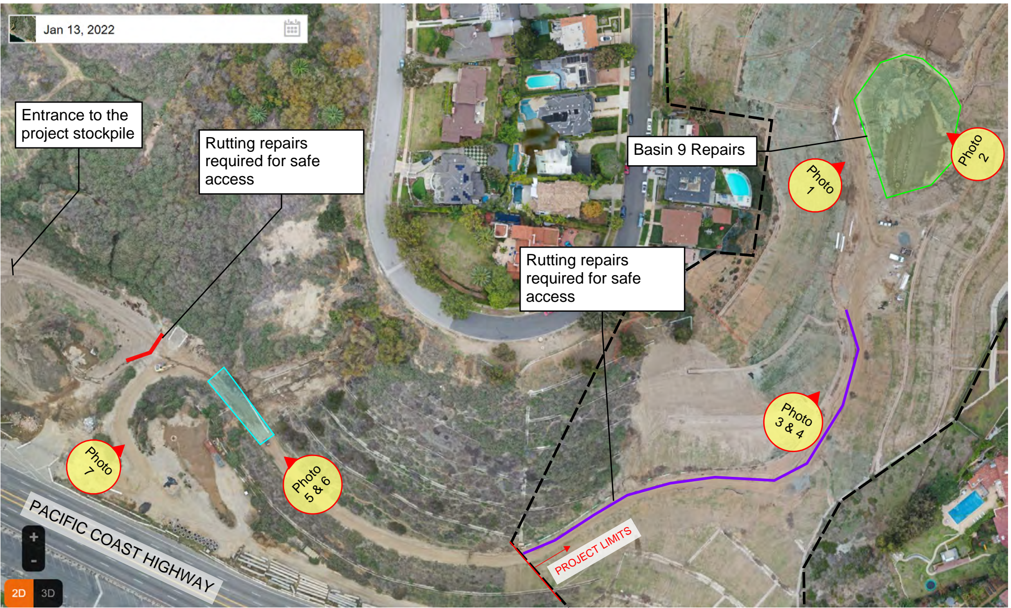
Figure 2: Main areas of significant damage sustained from the December 2021 storms located in the lower portion of the park.
